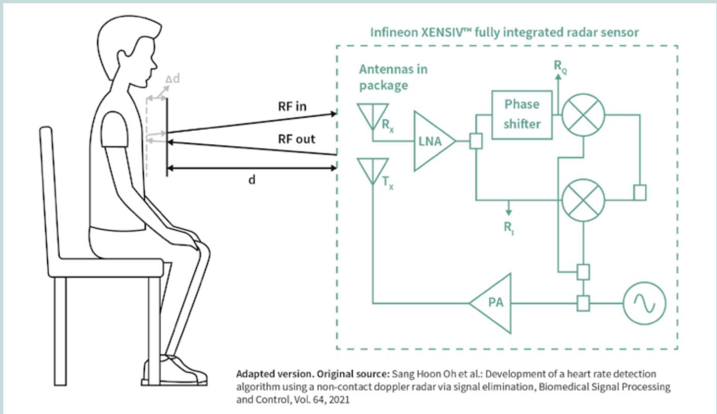
**Figure 2:** Operating principle of radar technology for vital sensing
